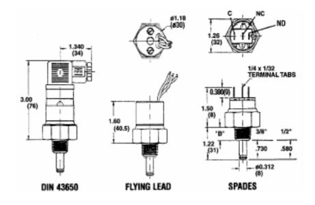
The PDTF is a factory set temperature alarm switch for protection of all types of internal combustion engines, pumps, compressors, gear boxes, hydraulic reservoirs, marine and industrial power plants.
